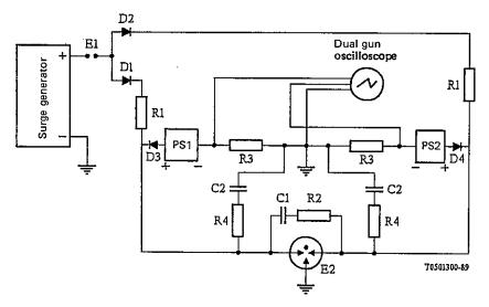
E1 Isolation gap or equivalent device
