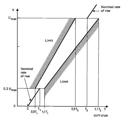
${\it Note} - {\it Spark-over}$  test waveform (nonconducting) must be within enclosed limits.
