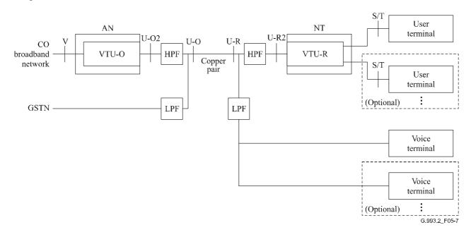
Figure 5-7/G.993.2 – Data with POTS service application model for remote deployment with splitter
