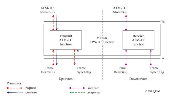
Figure K.6/G.993.2 – Signals of the VTU-R ATM-TC function
