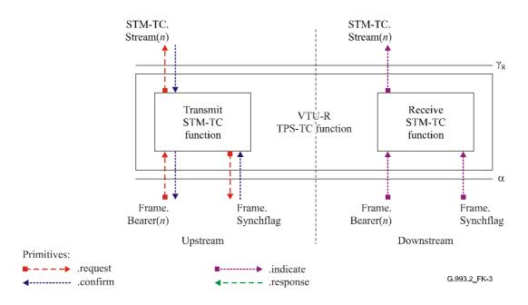
Figure K.3/G.993.2 – Signals of the VTU-R STM-TC function
