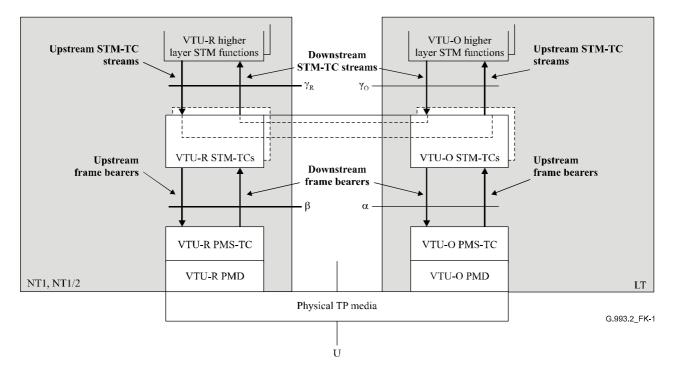
Figure K.1/G.993.2 – STM-TC transport capabilities within the user plane
