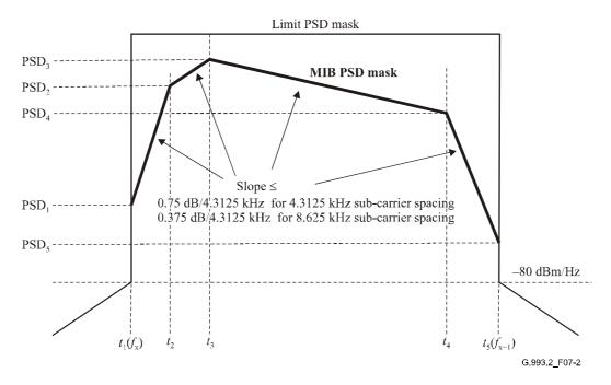
Figure 7-2/G.993.2 – Illustration of a MIB PSD mask in the case all breakpoint PSD<sub>n</sub> values are greater than -80 dBm/Hz
