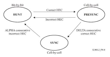
Figure K.9/G.993.2 – Cell delineation procedure state machine
