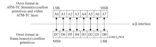
Figure K.8/G.993.2 – Bit mapping of the user plane transport function of the ATM-TC function
