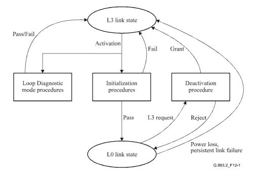
Figure 12-1/G.993.2 – VDSL2 link state and activation/deactivation procedures diagram
