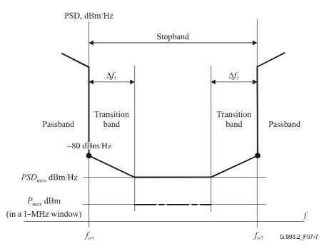
Figure 7-7/G.993.2 – Limit PSD mask and wide-band power limit in the stopbands
