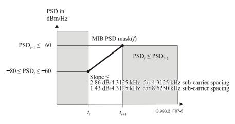
Figure 7-5/G.993.2 – Illustration of the one-slope steep upward shape
