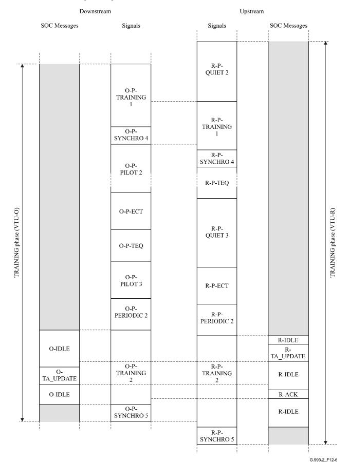
(see 12.3.4.3). The two outer columns show the messages that are sent over the SOC (see 12.3.4.2). The shaded areas correspond to periods of time when the SOC is in its inactive state.
