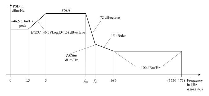
Figure A.3/G.993.2 – VTU-R US0 transmitter PSD mask for all-digital mode operation
