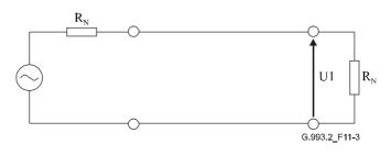
Figure 11-3/G.993.2 – Voltage across the load
