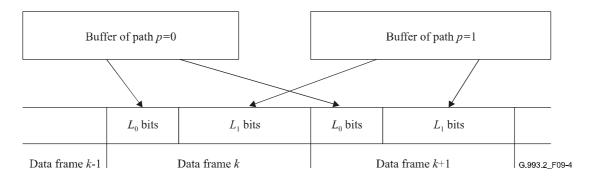
Figure 9-4/G.993.2 – Multiplexing of two latency paths into data frames carried by DMT symbols
