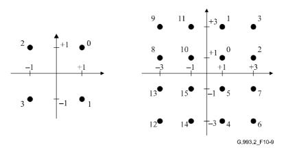
Figure 10-9/G.993.2 – Constellation labels for b = 2 and b = 4
