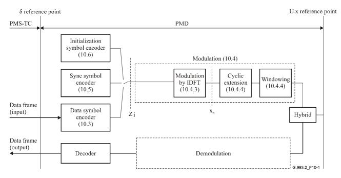
Figure 10-1/G.993.2 – Functional model of PMD sub-layer
