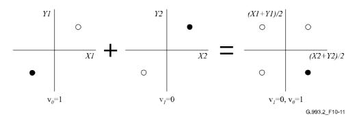
Figure 10-11/G.993.2 – Combination of a pair of 1-bit constellations to build a 2-bit constellation
