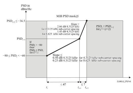
Figure 7-6/G.993.2 – Illustration of the two-slope steep upward shape
