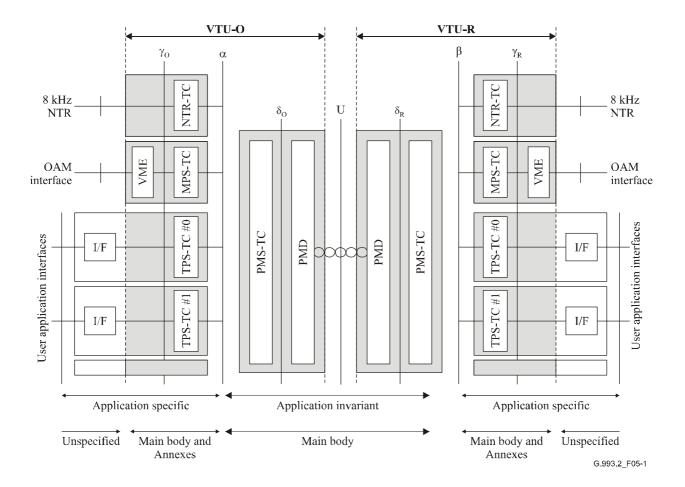
Figure 5-1/G.993.2 – VDSL2 and VTU functional model
