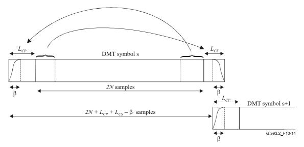
Figure 10-14/G.993.2 - Cyclic extension, windowing and overlap of DMT symbols
