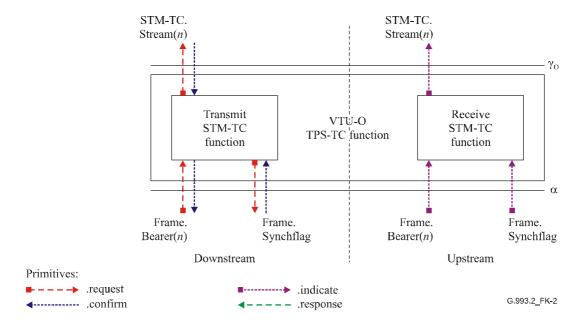
Figure K.2/G.993.2 – Signals of the VTU-O STM-TC function
