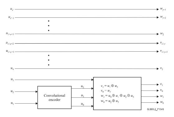
Figure 10-5/G.993.2 – Conversion of *u* to *v* and *w*
