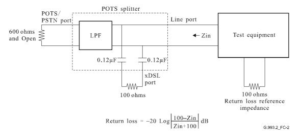
Figure C.2/G.993.2 – Impedance measurements in the band between 12 MHz and 30 MHz for the CO and remote POTS splitters
