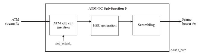
Figure K.7/G.993.2 – Block diagram of transmit ATM-TC function
