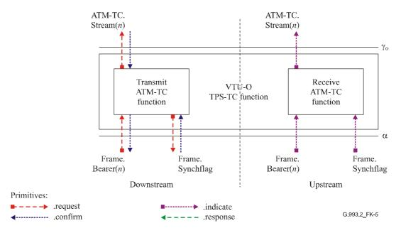
Figure K.5/G.993.2 – Signals of the VTU-O ATM-TC function
