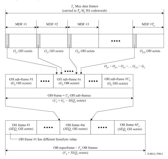
Figure 9-3/G.993.2 – Overhead sub-frame, frame, and superframe structure
